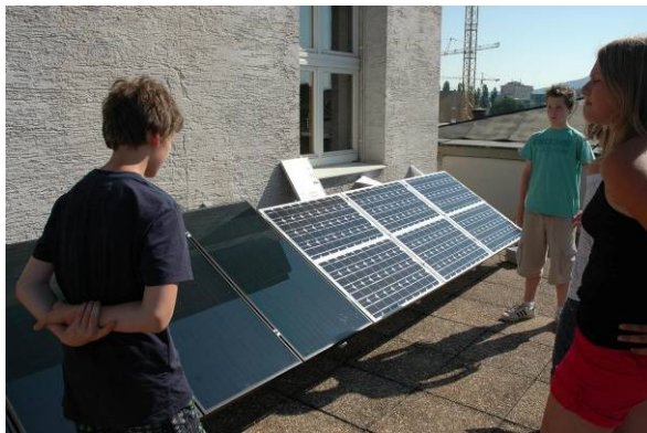
Station PV-Forschungsanlage – Module (monokristallin / CIS)
